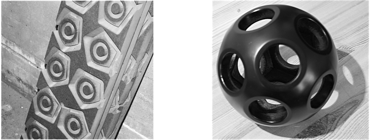
Figure 3.9: left: The milled MDF board with the segments after the CNC-machine; right: The finished cabinet
