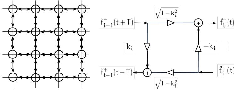
Figure 62: *left figure* – Scheme of a digital waveguide mesh in two dimensions.
