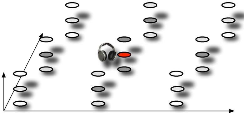
Figure 58: Schematic plot of the data listening space. Three space-like dimensions of the QED lattice are placed virtually in a real physical space. A listener can move freely about with headphones that are tracked with infrared cameras. Each dot represents the virtual position of a sound in the data listening space. The positions in the height dimension are compressed.
