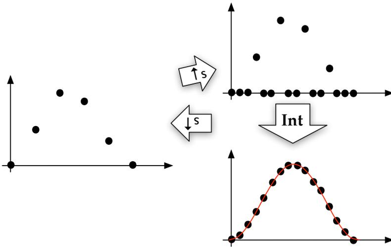
Figure 48: Up-, down-sampling, and interpolation. The factor of the sampling in the example is  $s = 3$ . The red curve shows the perceived function. The x-axis shows time/samples, the y-axis the signal function.
