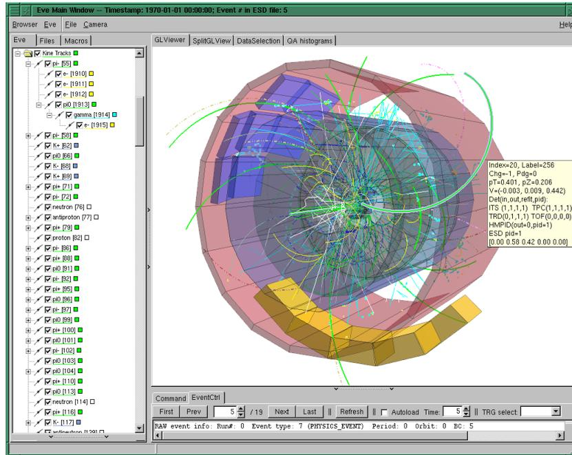
Figure 65: Screenshot of AliEve [TMT00], the visualization tool of the ALICE offline group. The reddish surface gives the volume of the TPC (yellow and blue are other detectors). Each line is the track of a particle of this event.
