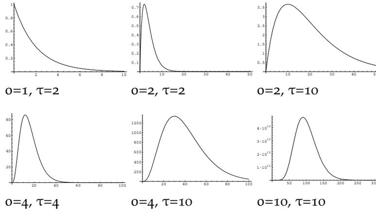
Figure 49: Envelope function proportional to the gamma distribution, Eq. (5.10). For  $o = 1$ , the attack time is 0;  $o > 1$  controls the ‘order’ of the attack time.  $\tau$  controls the decay time (note that the running index  $t$ , shown on the x-axis, as well as the maximum ordinate value, change in scale!).
