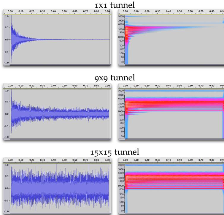
Figure 64: Examples of a  $20^3$  sites waveguide mesh, excited with an impulse (all values set to one) at time  $t = 0$ , and run for 20,000 samples. Three percolating tunnels of different sizes were programmed into the mesh as ‘test clusters’. Small tunnels lead to the excitation of higher frequencies, and lose their energy quicker than large tunnels, which excite also low frequencies, due to longer distances of free wave propagation between adjacent (hard reflecting) cluster sides.
