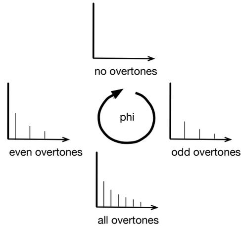
Figure 67: Simplified scheme of the overtone structure in the TPC sonification depending on the angle  $\phi$ . The overtone structure helps disambiguating the correct grouping and separation for single sounds into coherent tracks, even if these tracks have similar pitches.
