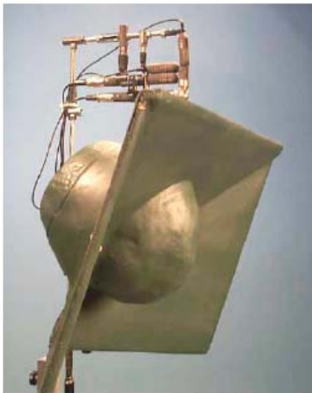
Fig. 9 - New design of the PanAmbiophone. Two pairs of small pressure microphone elements are coincident at 'ear' positions. A discrete soundfield array is mounted atop – a total of eight recording channels for PerAmbio 3D (with height).
