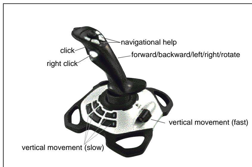
[Fig 18] Joystick with input possibilities
