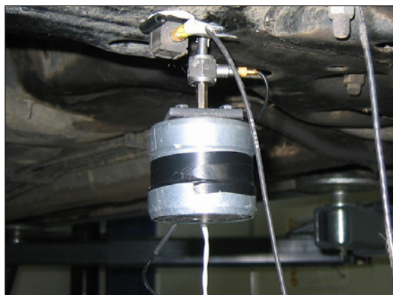
Fig. 3: Shaker and force transducer fixed to chassis using X60 glue.
