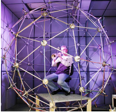
Figure 1: Surrounding microphone array (Hohl [7]) with 64 channels.
