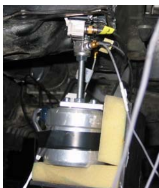
Figure 4: Measurement setup for one excitation position including Mini Shaker, force transducer and accelerometers
