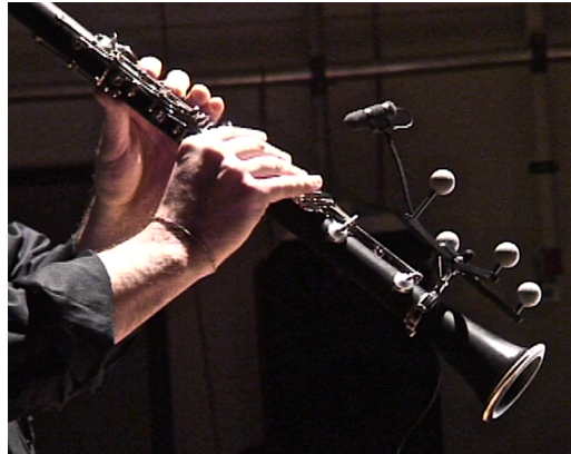
Figure 1. A 4-marker tracking target mounted on a clarinet using a Marschgabel fitting (and microphone attached)
