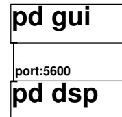
Figure 2: Pd as it usually operates: the pd-gui process connects to the engine ( pd dsp ) on (e.g.) port 5600.
