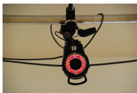
Figure 3: Infrared camera of the VICON motion tracking system.
