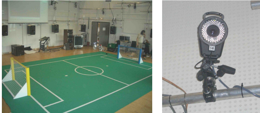
Fig. 1: The experimental setup for the data recording. The left image shows the RoboCup Standard Platform League field within motion capturing system. The right image shows one of the 15 cameras of the body motion tracking system. The LEDs at the front of the camera provide pulsed infra-red light allowing capturing under day light conditions.
