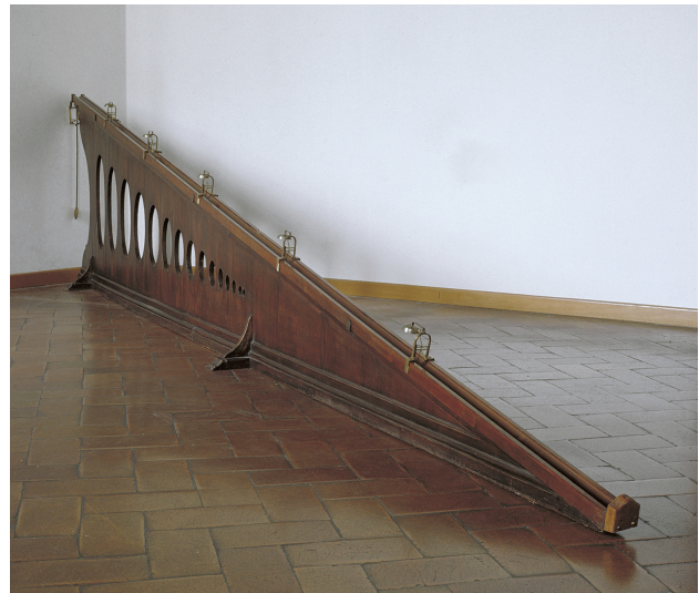
Figure 1: Experimental device of Galileo Galilei for experiments of the law of falling bodies. In rolling down the inclined plane, the ball hits the bells which are attached following a quadratic law. The resulting rhythm is regular. This device is rebuilt at the Istituto e Museo di Storia della Scienza in Florence. ©Photo Franca Principe, IMSS, Florence.
